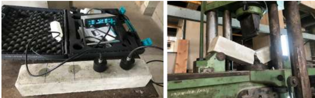
Figure 5: (a) Ultrasonic Pulse Velocity Testing (UPV) on the beam (b) Flexural strength test on the beam with centre-point loading.
